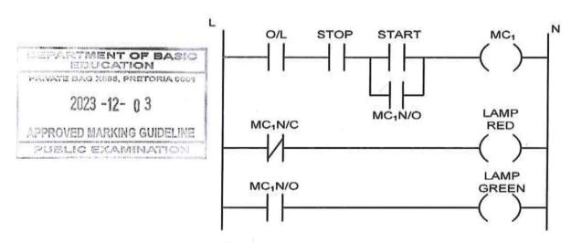
NOTE: It will also be accepted if both the O/L and STOP symbols are closed. NB, both O/L and STOP must be the same state. (9)
