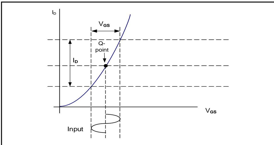
**FIGURE 4.2: CHARACTERISTIC CURVE**
