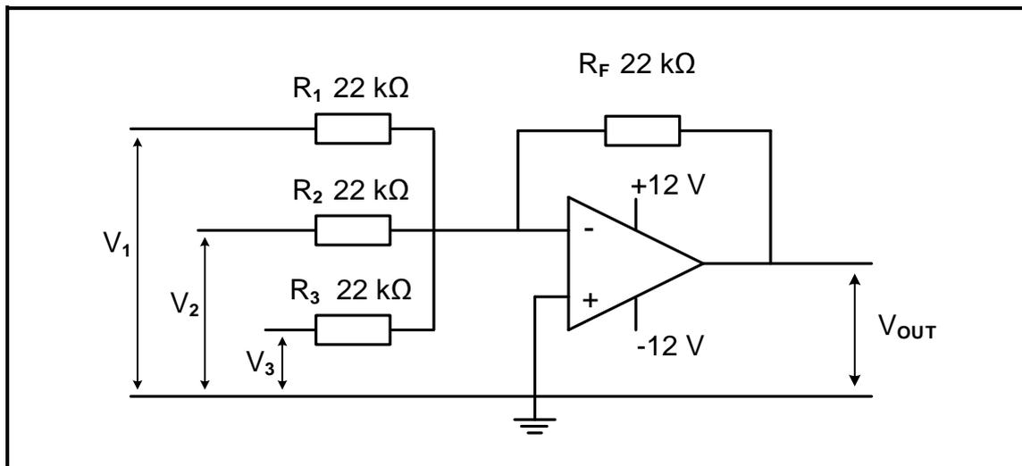
**FIGURE 5.7: OP-AMP CIRCUIT**
