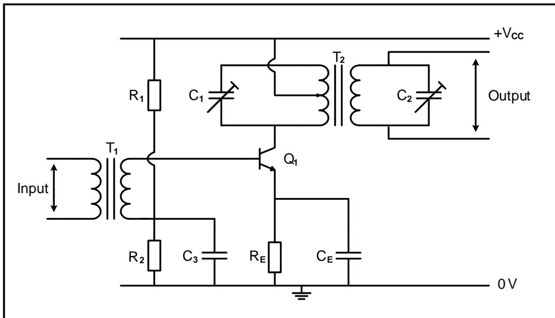
**FIGURE 6.5: RADIO-FREQUENCY AMPLIFIER**
