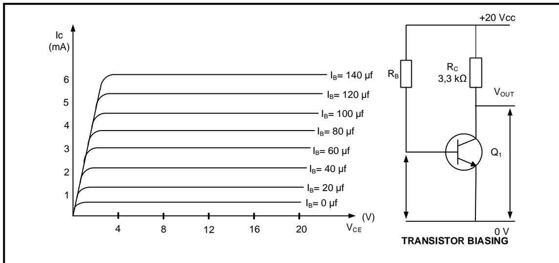
**FIGURE 6.2: CHARACTERISTIC CURVE OF A TRANSISTOR CIRCUIT**
