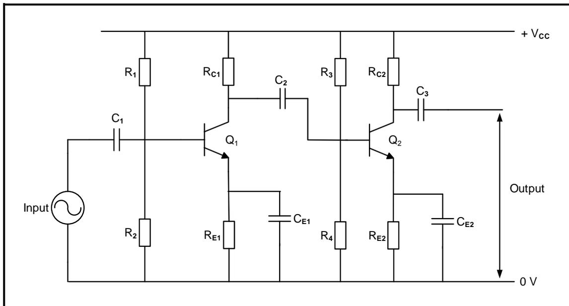
**FIGURE 6.3: TWO-STAGE RC-COUPLED AMPLIFIER**
