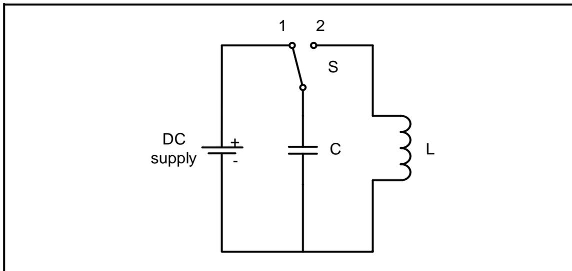
**FIGURE 6.6: TANK CIRCUIT**
