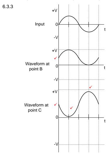
NOTE: 1 mark for DC offset and duplicate of the input at B
