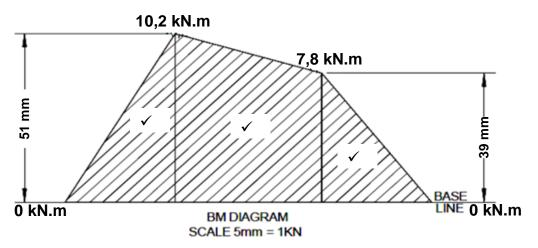
Markers need to draw to scale at marking centre SCALE 5mm =1kN.m
