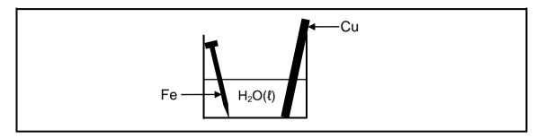
After a while it was observed that the iron nail was coated with rust. The copper rod showed no visible signs of corrosion.
