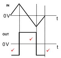
1 mark for phase shift 2 marks for correct orientation
