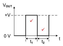
4.3.3 If the value of R₁ is increased, the RC time constant of the charging circuit (t₁) increases, ✓ keeping the output of the 555 IC high for longer. ✓ This means that the positive output pulse (high) will be longer than the negative output pulse (low). ✓
