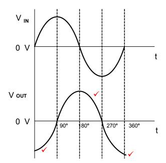
1 mark for 90° phase shift Correct orientation of which will be:
