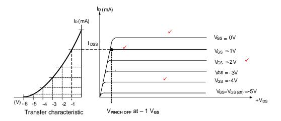
**NOTE**: 2 marks for the family of curves 1 mark for the range of V<sub>GS</sub>
