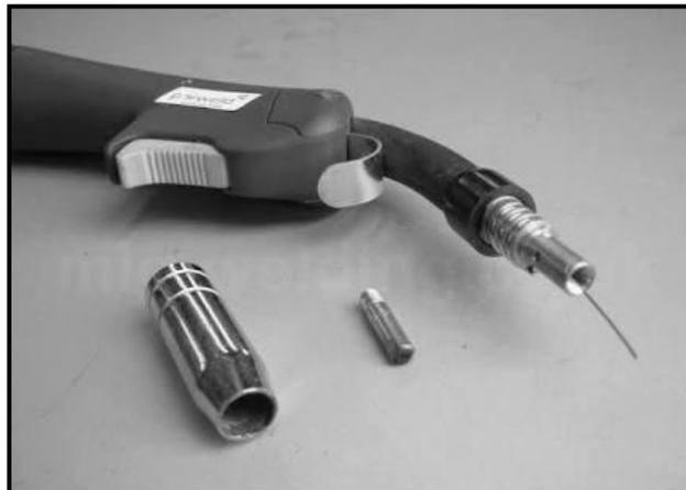
4.3.1 Describe the process when replacing a worn welding tip. (4)
