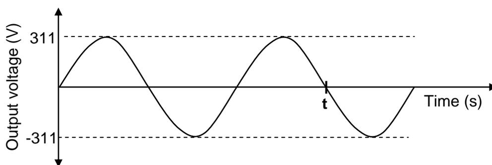
The output voltage is generated at a frequency of 50 Hz.
