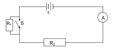
Which ONE of the following combinations about the ammeter readings will be CORRECT when switch S is open and when switch S is closed?
