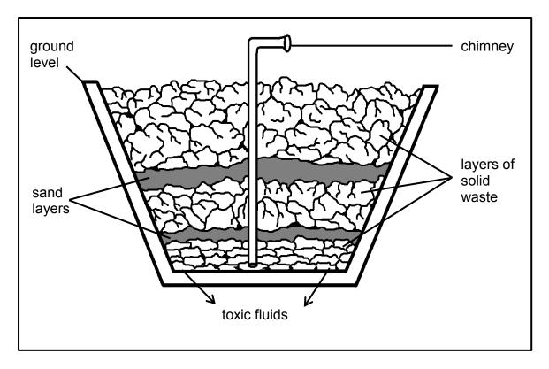
2.2.1 Name the flammable gas that escapes through the chimney. (1)
